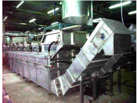
Figure 3.23. Sink-float tank in a PET bottles recycling line (Courtesy of OCI GmbH)
